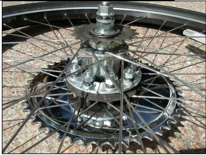
Figure -2 9 slot - Chain Wheel Sprocket Installation mounted dish side inward
