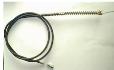
Push button Clutch lever - Dual lever Clutch & Brake Clutch cable end barrel locks in lever handle.
