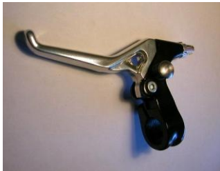
Push button Clutch lever - Dual lever Clutch & Brake Clutch cable end barrel locks in lever handle.
