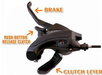
Push button Clutch lever - Dual lever Clutch & Brake Clutch cable end barrel locks in lever handle.
